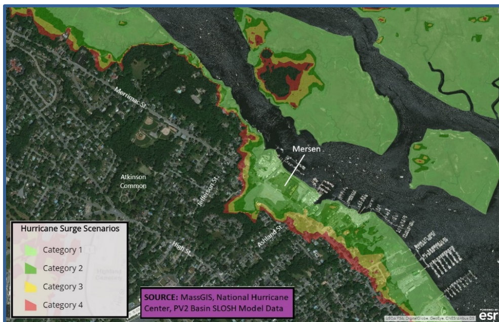
Figure 91. Hurricane Storm Surge Inundation – Mersen Area
