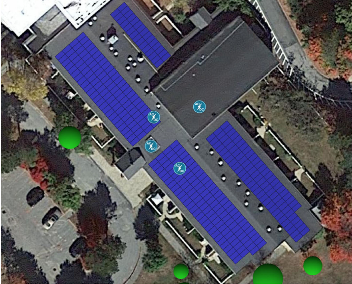
Figure 2: Location 1.1 Panel Layout – Rooftop.
