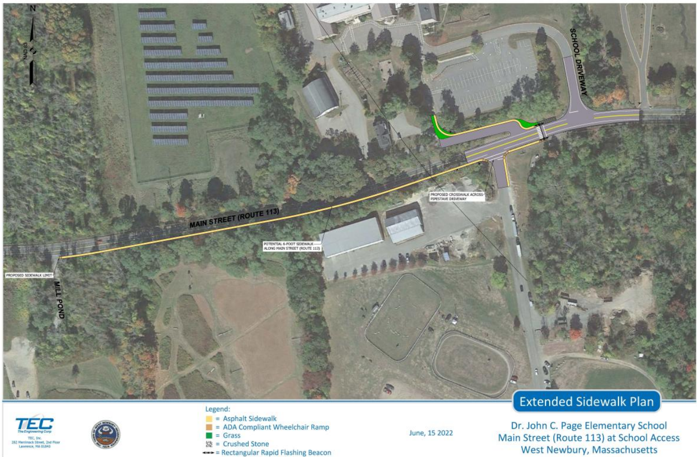
Above: Broader geographic scope of November 2022 Safe Routes to Schools application called for new sidewalk along Route 113, in addition to improved crossing and RFB at Page/Pipestave
