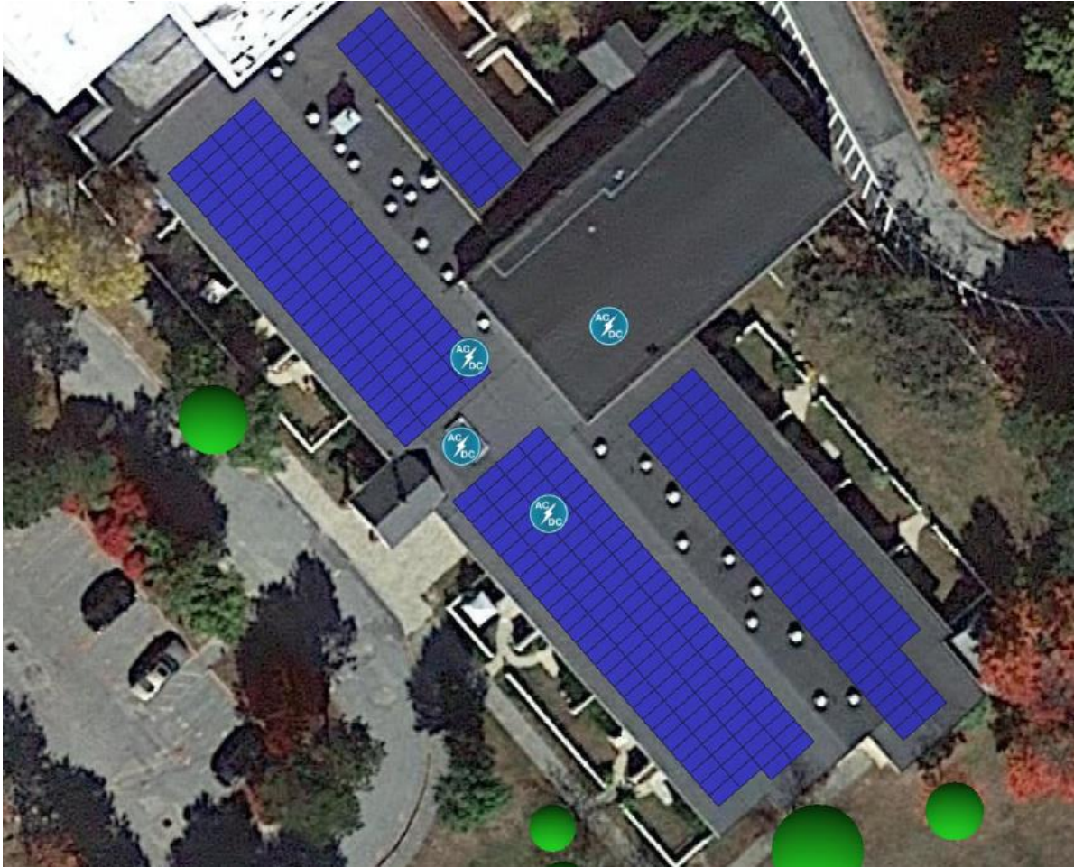
Figure 2: Location 1.1 Panel Layout – Rooftop.
