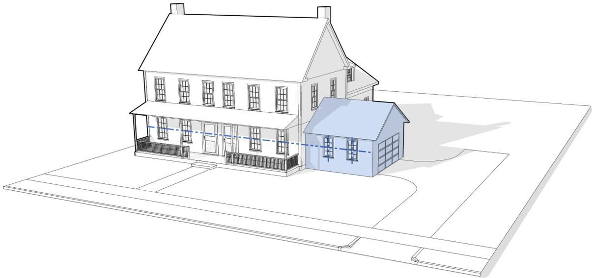
ii. When located on the front façade of a building, a garage must be set back at least 2 feet from the front façade (A). A front-facing garage door may be no wider than 12 feet (B). Front-facing garage doors shall occupy no more than 1/3 of the front façade of a building (B/C). At least twenty (20) linear feet of backing space (D) must be provided between a garage and a sidewalk or street edge (whichever is less), unless the garage is accessed from an alley.
