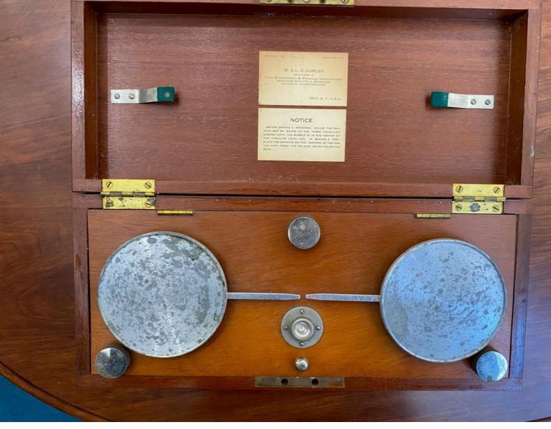
Portable scale owned by the West Newbury Department of Weights and Measures whose instructions ask the user to "adjust the balance box by means of the three leveling screws until the bubble is in the center" to
